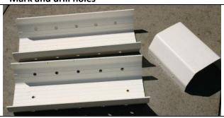
Mark and drill the ventilation holes. They are about 7mm across. You need to strike a balance between not letting the rain in, not creating wind chill, and allowing the air to circulate. Mark and drill smaller holes to attach the piano hinge with. You will also need two holes on the back for hanging the weather station on a post.
