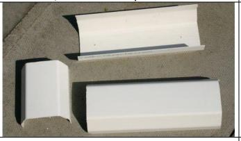
The front and back are made from lengths 30cm long. Check what is needed for your thermometers. The roof section is
