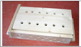
Fill screw holes. Paint with primer, undercoat and top coat. The final coat must be white gloss to reflect the heat of the sun.
