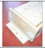
Drill 16mm ventilation holes in sides, front and base. These are at 5cm intervals. Avoid screws.
